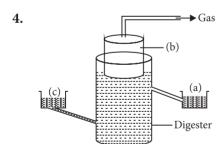
The diagram above is that of a typical biogas plant. Explain the sequence of events occurring in a biogas plant. Identify a, b and c.
